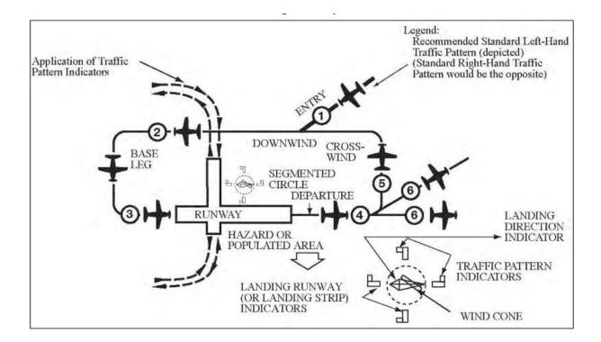
Shown above is the traffic pattern schematic as shown in the AIM. The only leg missing is the Upwind Leg, which is also the departure leg 3.
