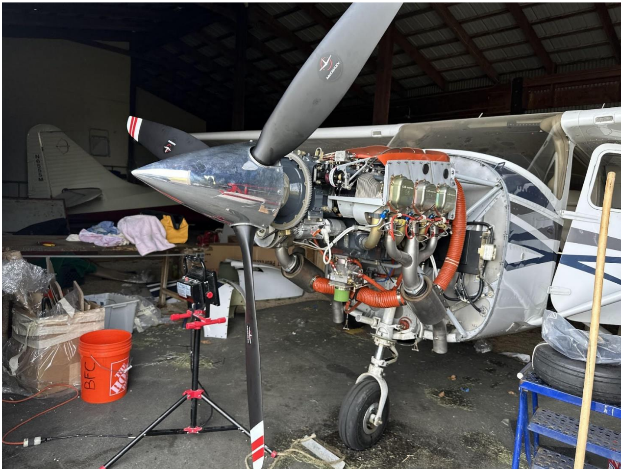
The rebuilt engine mounted on the 182
