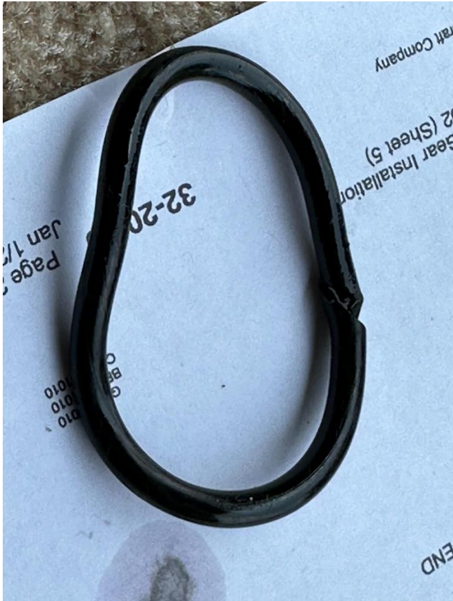
The failed nose strut gasket
