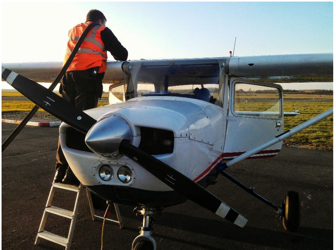
Correct fueling technique, leaves no black marks. Leave yourself extra hose slack.
