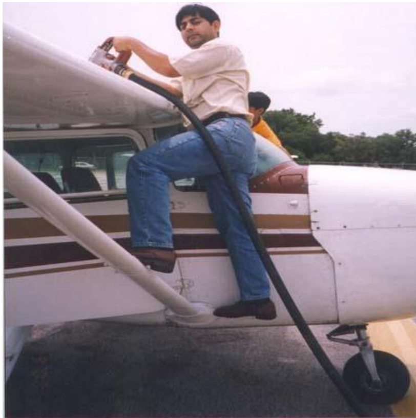
Incorrect fueling technique leaves black marks on the leading edge.
